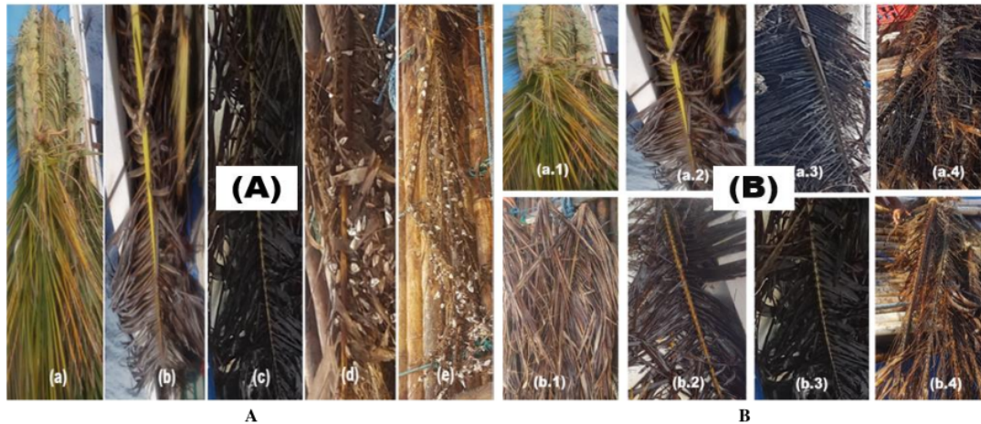
Figure 3. A. The average physical changes of coconut leaves attractor. (a). Condition before immersion in the sea, (b). 1-2 weeks old, (c). 3-4 weeks old, (d). Age 5-6 weeks, (e). Age 7-8 weeks; B. Durability of coconut leaves attractor during submersion in the sea based on usage. (a.1). Fresh/green leaves (b.1). Dried leaves/brown
